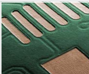
Creation of solder mask openings
